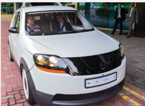
TUM CREATE and NTU developed EVA, an electric car designed as a taxi for tropical megacities.
