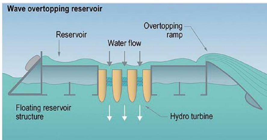
Figure 6: an example of wave energy technology: overtopping converters
