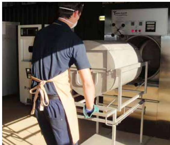
DEMONSTRATING THE MEDI-CLAVE AUTOCLAVE TECHNOLOGY DESIGNED FOR SUB-SAHARAN AFRICA UNDER THE GEF/UNDP/WHO/HCWH GLOBAL MEDICAL WASTE PROJECT. PHOTO BY JORGE EMMANUEL.
