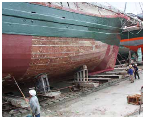
SHIP YARD WORKERS APPLYING DDT-FREE ANTI-FOULING PAINT ON THE HULL OF A VESSEL IN YANGJIANG CITY, GUANGDONG PROVINCE. PHOTO BY MS. SHI SHENGNAN. THE FOREIGN ECONOMIC COOPERATION OFFICE (FECO).
