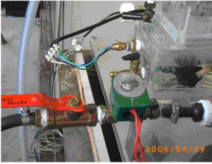
Figure 1. Air compressor (top) and solenoid valve (bottom).
