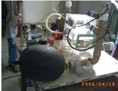
Figure 2. The air heating and humidification system prototype coupled to a fully blown rubber made test lung.
