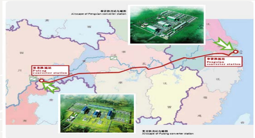
Xiangjiaba (Southwest China)-shanghai \pm 800 kV UHVDC grid
