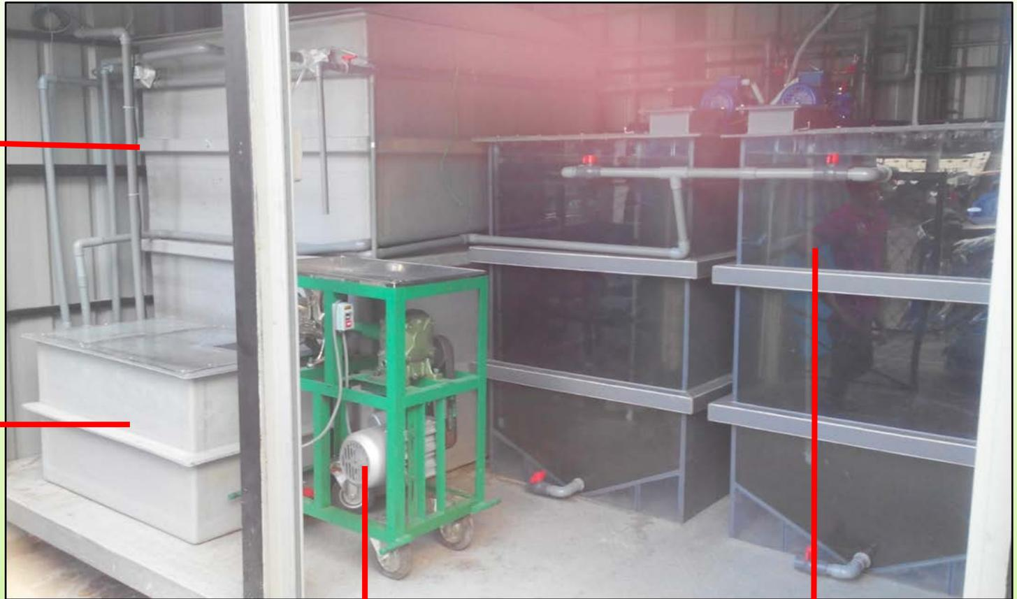
Grinder to grind the food waste – faster the digestion process
