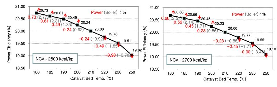
Power Generation Efficiency according to NCV and Catalyst Bed Temp. Changes
